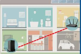
Why does this happen? The MVlilnk GigaSpire router is designed to be a mesh unit as well (to extend Wi-Fi coverage) and looks for other devices on the network. So, when the GigaSpire detects the third-party router, it shuts
