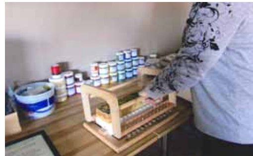
Lorna demonstrates how the cutter is used to make the bars of soap equal in size.
